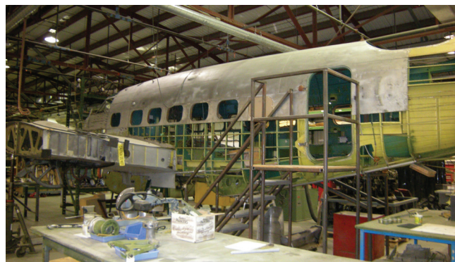
FK466 fuselage restoration, with wings and tail from Lockheed CF-CEC added. Photo Courtesy - NAFMC
