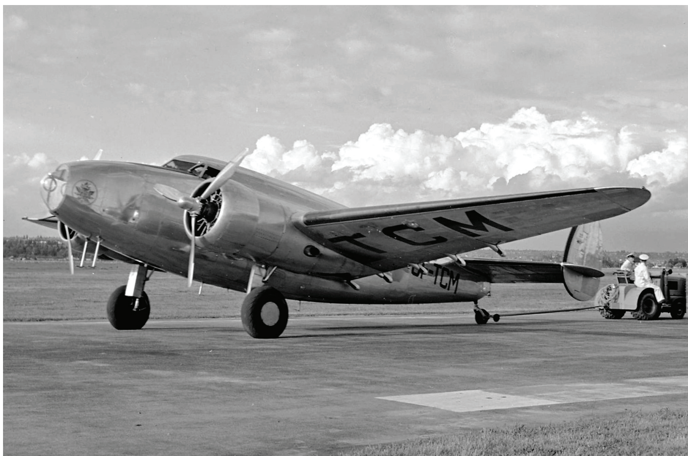
TCA's CF-TCM Lockheed Super Electra Model 14 - This design was developed into the Hudson Bomber. Photo Courtesy - TCA- Air Canada
