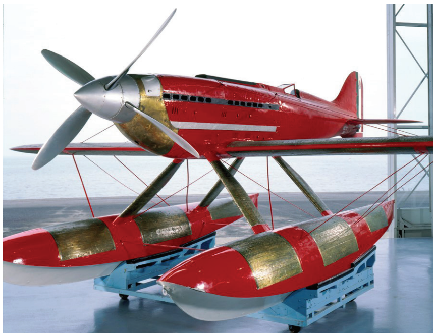
The Macchi - Castoldi M.C.72 at the Italian Air Force Museum near Rome. The Oil Radiators are visible in the pontoons.
