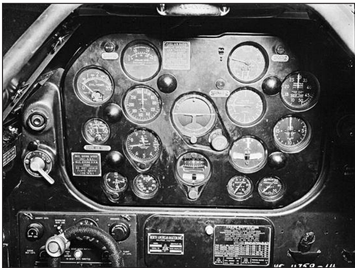
The front cockpit main instrument panel of an RCAF Harvard Mk.II, circa 1941. That for the same mark in 1954 was practically identical.
