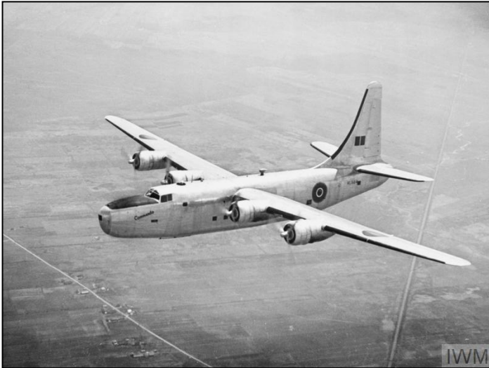
RAF Consolidated LB-30 Liberator Mk. II, AL504, Commando , in flight over Canada, November 1944. This was after the aircraft was converted from a double fin tail to single fin. ©www.iwm.com
