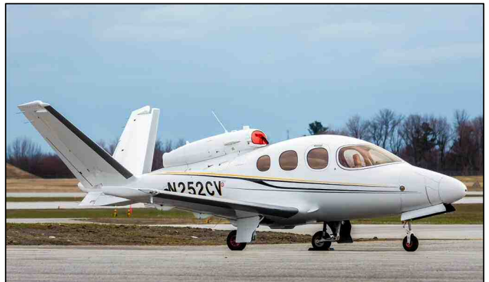
This Cirrus Vision SF50 (c/n 0004), N252CV, is one of a new breed of Very Light Jet (VLJ) single-engine aircraft. Developed by Cirrus Aircraft at Duluth, Minnesota, the Vision was FAA certified in October 2016 and has 600 orders at nearly US$2 million per copy. Powered by a single Williams FJ33-5A turboprop, it carries 1 pilot and 6 passengers at a cruise speed of 300 knots.
