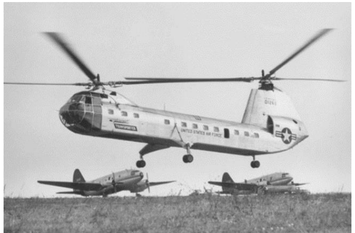
The U.S. Air Force prototype Piasecki YH-16A Transporter. The program was abandoned after the crash of the second prototype. © U.S. Air Force photo from the USAF Aeronautical Systems Center History Office, Public Domain.
