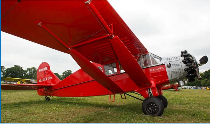
Big Sky Stearman's 1929 Bellanca CH300 (c/n 133) Pacemaker, NC688E, with its 420-hp Wright R-975-11 Whirlwind engine.
