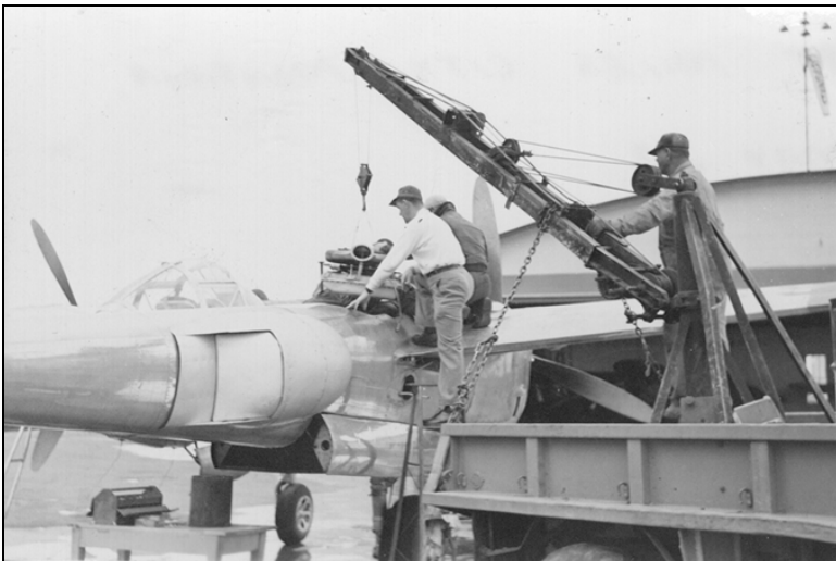
Changing the Turbo Charger on a P-38, Miles City, Montana, 1953
