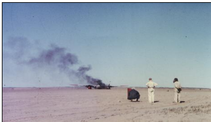
Mosquito Mk 35 belly lands at Pelly Lake after engine failure. Aircraft totally destroyed, crew uninjured.
