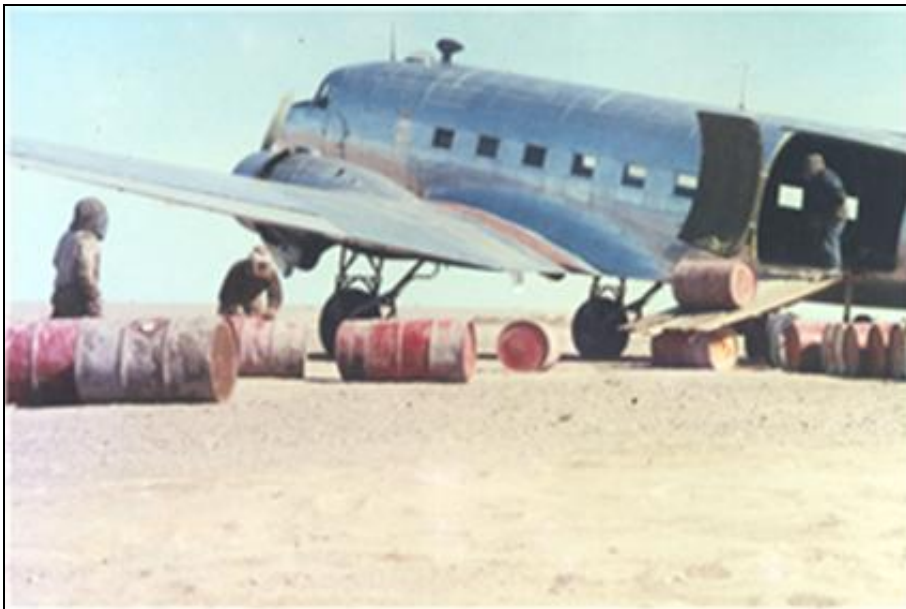
Unloading fuel at Pelly Lake, NWT. The DC-3 flew in nine drums per trip. ©Syd Baker
