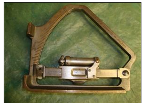
Sydney Baker's Clinometer Field Mark III No. 6913, Circa 1915 Mfr. CSI Co. Ltd. Cambridge. (C Hine photo)
