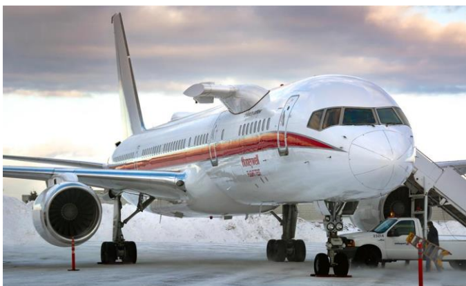
This unusually configured Boeing 757-225, N757HW (c/n 22194) made an overnight stop on January 14 th whilst en route to the UK. The aircraft is operated by Honeywell as a flying engine test bed. Test engines are carried on a pylon on the right side of the forward fuselage. © Ben Senior
