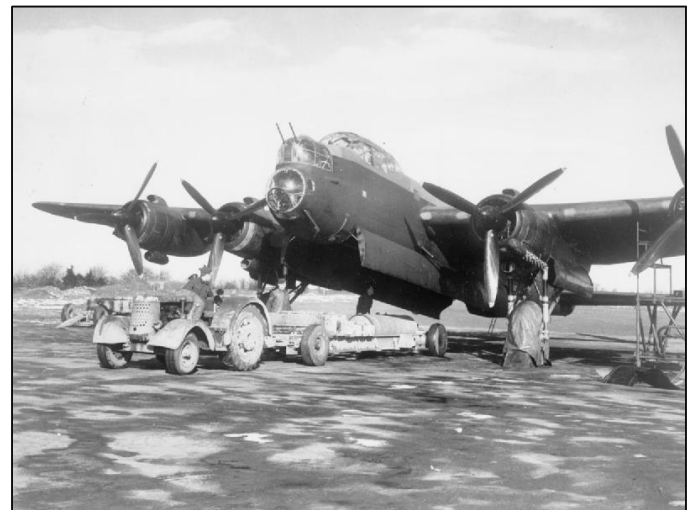
Avro Lancaster B Mark II, LL725 'EQ-C', of No. 408 Squadron RCAF, on the ground at Linton-on-Ouse, Yorkshire. Armourers are backing a tractor and trolley loaded with a 4,000 lb HE bomb ('Cookie') and incendiaries under the open bomb-bay. LL725 was lost over Hamburg on 28/29 July 1944. (© RCAF)
