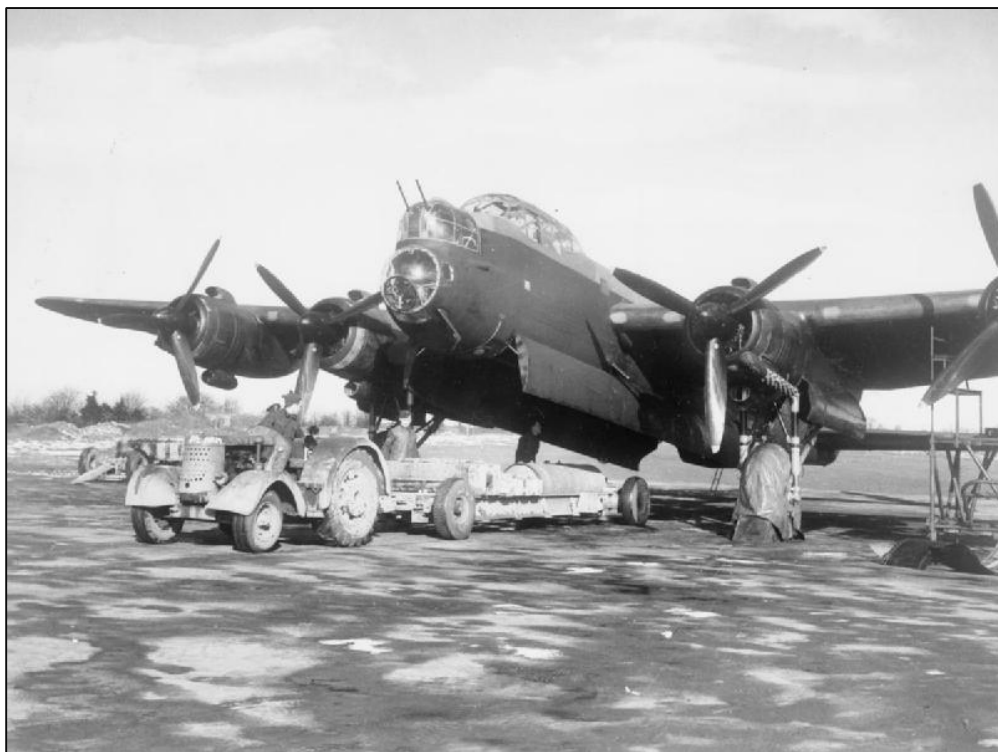
Avro Lancaster B Mark II, LL725 'EQ-C', of No. 408 Squadron RCAF, on the ground at Linton-on-Ouse, Yorkshire. Armorers are backing a tractor and trolley loaded with a 4,000 lb HE bomb ('Cookie') and incendiaries under the open bomb-bay. LL725 was lost over Hamburg on 28/29 July 1944.
