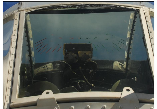
Liberator GR. VIII 11130 rear gun turret close-up showing graduation markings (© Bill Upton)
