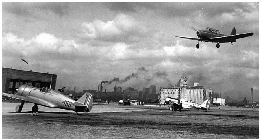
Little Norway Toronto Aircraft L-R - Curtiss P-36 - Douglas DB8A-5 - Fairchild PT-26 - Photo Credit - forsvretsmuseer.no
