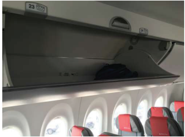
The CS100 has larger and five inches lower overhead bins and enlarged oval windows.
