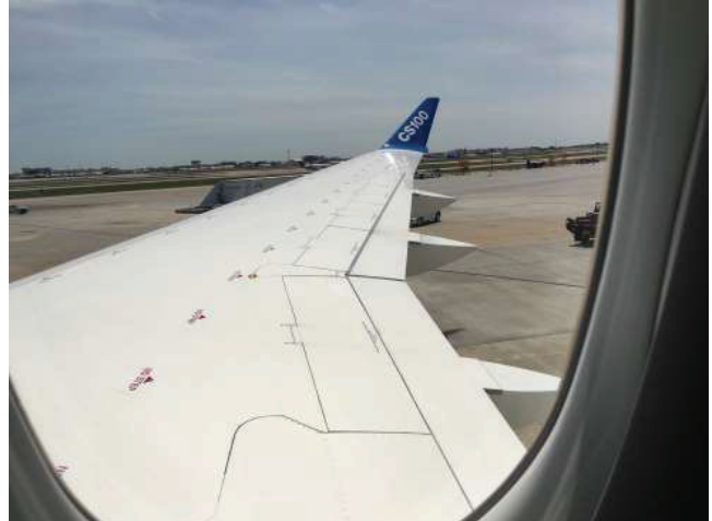
The CS100 has been certified for operation into the London City Airport 4000 foot runway due to the large wing and high lift devices.
