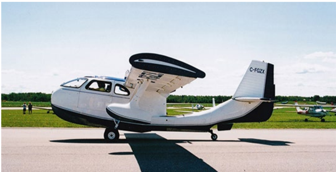
Republic RC-3 Seabee, C-FGZX, restored as a Beeboyz Seabee with a GM LS2 engine, arriving at Edenvale Aug. 13, 2017.
