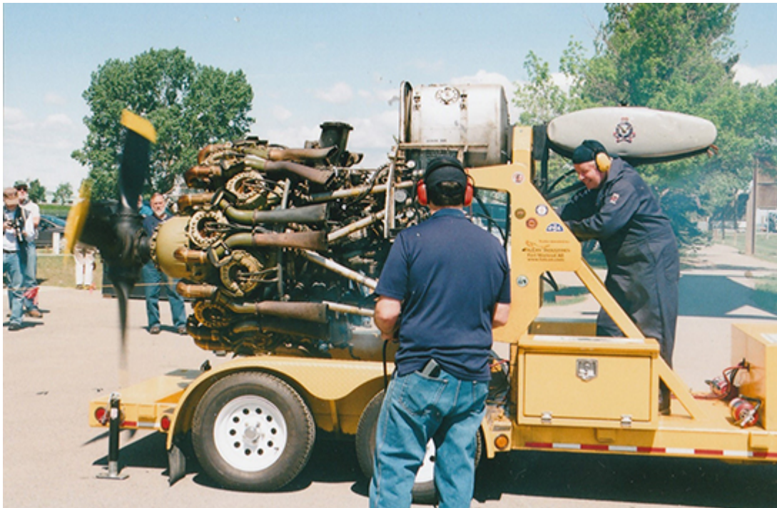
Karl Kjarsgaard fires up a 1,650 hp Bristol Hercules engine at the Bomber Command Museum for convention attendees. (G. McNulty photo)
