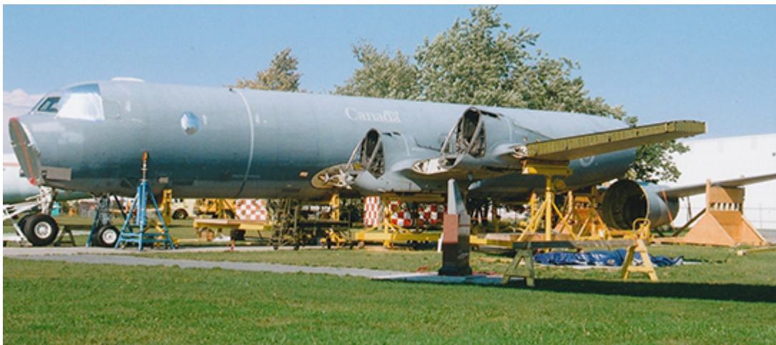
Lockheed CP-140 Aurora 140102 being reassembled at NAFMC.
