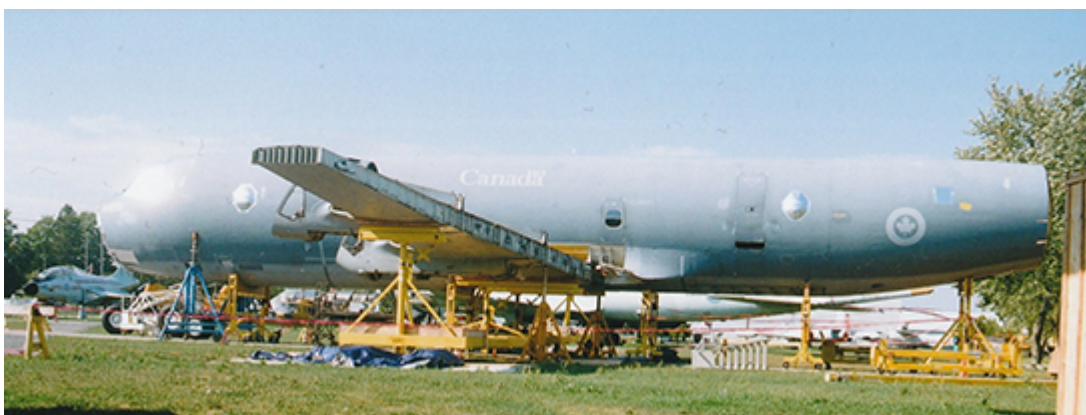
Lockheed CP-140 Aurora 140102 being reassembled at NAFMC.
