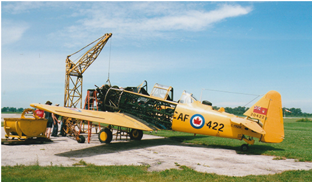
CHAA volunteers remove the engine from a Harvard Mk 4 during the 80 th Anniversary celebration.
