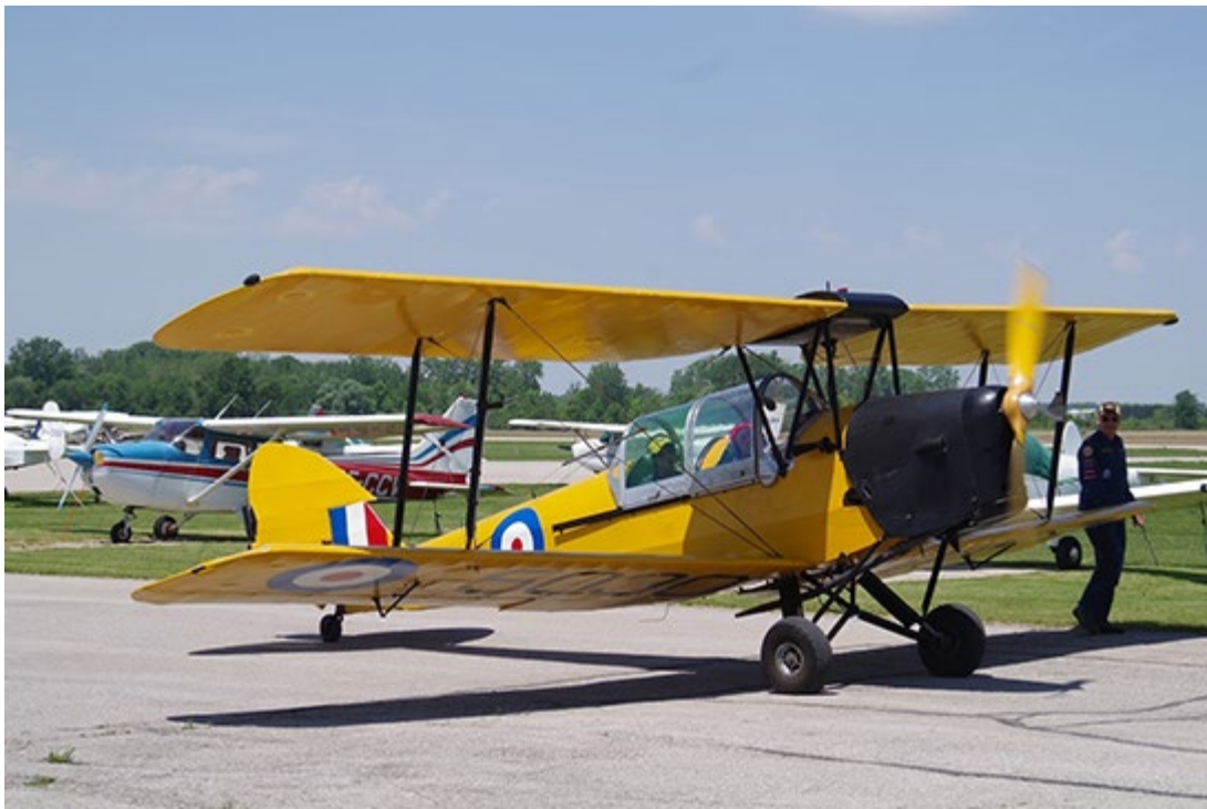
Tiger Moth 5030 needed a wing walker to keep straight in the breeze while taxiing back to the apron after a flight.
