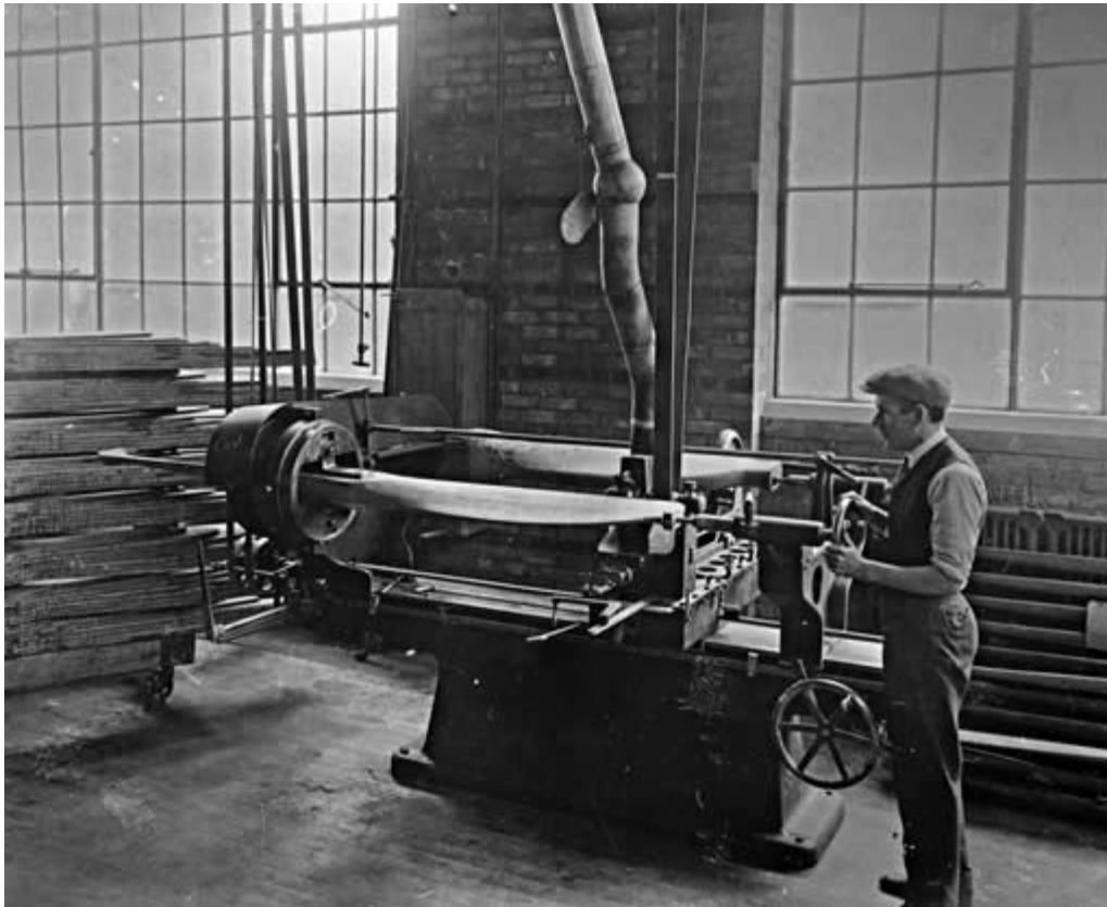
Curtiss JN-4 "Canuck" propeller on turning lathe at Canadian Aeroplanes Limited factory, Toronto Ontario 1917-1918. Source: Canadian Aviation Through Time
